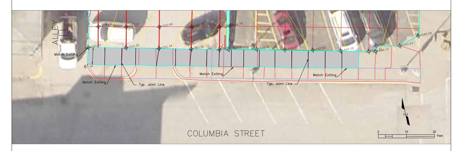
Contractor to remove existing concrete. Excavate approximate 3" of material and place new granular subbase. Place new concrete at a depth of 5 inches. Match into adjacent existing concrete. Dimension of sidewalk is approximate 6 feet by 97 feet.
